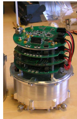
Fig. 15. Avionics module developed by SF for the scaled model of PERUN demonstrator rocket
