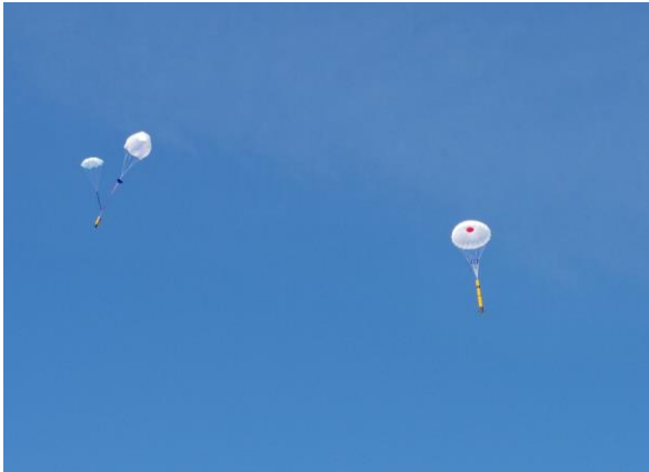
Fig. 9. Parachute deployment for the BIGOS 3 rocket developed by SF
