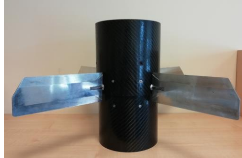
Fig. 14. Canards guidance module developed by SF for the scaled model of PERUN demonstrator rocket
