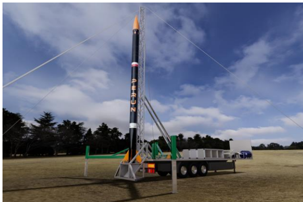
Fig. 18. Rendering of the TEL in its launch configuration
