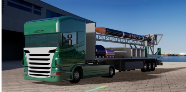
Fig. 17. Rendering of the TEL during transportation configuration
